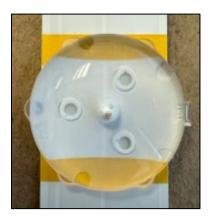
23. The '162 Patent Accused Products comprise a transparent dielectric solid of revolution with external surface area predominantly comprised of an entry surface that receives light of nonuniform irradiance from a nearby compact light source and of an opposing exit surface that forms from said received light a pre-specified diverging output beam, as shown for example in the images from the QN65Q80CAF model television below.
