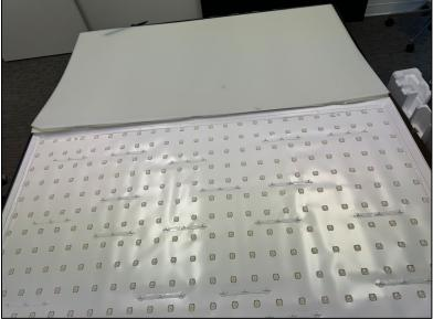
90. The '952 Patent Accused Products include a diffusion plate comprising a top surface and a bottom surface, such as the example shown in QN65Q80CAF model television below. The bottom surface is shown in the image and the top surface is the opposing side.
