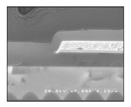
74. The '626 Patent Accused Products include light emitting devices made by sequentially forming an N-type semiconductor layer, active layer, and P-type semiconductor layer on a substrate as shown in the image below from the QN65Q80CAF model television.
