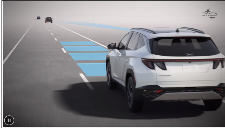
Forward Collision-Avoidance Assist with Pedestrian Detection (FCA-Ped) When the system detects a vehicle or pedestrian in your path, it warns you of a potential collision. If you don't begin stopping in time, the system may automatically apply braking. ⓘ
