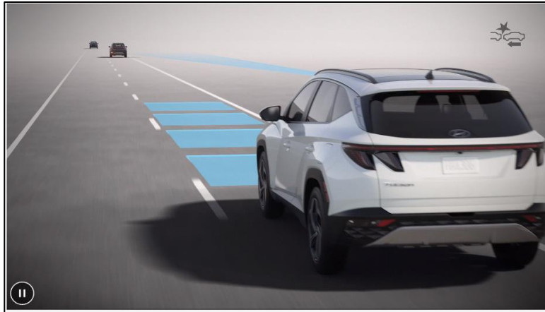
Forward Collision-Avoidance Assist with Pedestrian Detection (FCA-Ped) When the system detects a vehicle or pedestrian in your path, it warns you of a potential collision. If you don't begin stopping in time, the system may automatically apply braking. ⓘ
