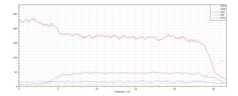
51. The below SIMS element trace analysis of Qorvo's QPD1000 Accused Product (done from the device's backside), along with the corresponding excerpt (highlighting added) of the underlying raw SIMS data used for the SIMS element trace analysis, shows that the Al signal (black in trace analysis and green in raw SIMS data) appears approximately 20nm before N (blue), while the Ga signal (magenta) appears approximately 10nm after N (blue).
