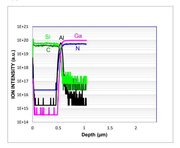
47. The below excerpt (highlighting added) of the underlying raw SIMS data used for the above SIMS element trace analysis shows that the Al signal (black in trace analysis and green in raw SIMS data) appears approximately 20nm before N (blue), while the Ga signal (magenta) appears approximately 10nm after N (blue).
