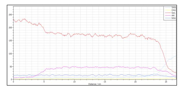
41. The QPD1000 Accused Product's SiC substrate is also indicated by the below SIMS element trace analysis (done from the device's backside), which shows the SiC substrate on the left-hand side (light-green and dark-green traces).
