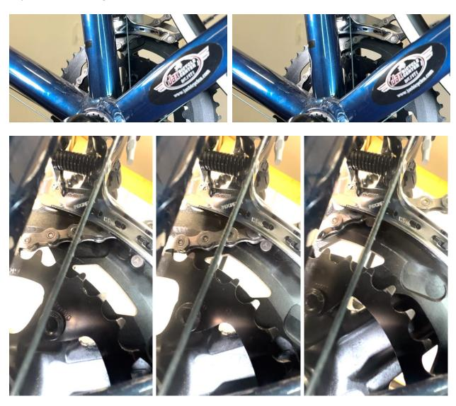
21. Each ramp has a ramp face on the inner surface of the chaining for receiving a link of an outside surface of a chain during an upshift.
