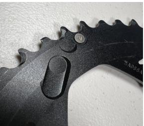
20. In normal operation, when upshifting from a smaller chaining, the derailleur moves the chain over to the inner surface of the larger rotating chaining, and the configuration of the ramps causes engagement of the ramp with at least one link of the bicycle chain at two or more distinct pivot points and lifts the chain toward the outer edge of the larger chaining, and the lifting is not assisted by (and precedes) engagement from any of the chaining teeth.
