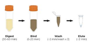
Simple, scalable, and quick protocol that is easy to adopt on any automation platform or on lab bench.
