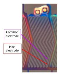
100. The products accused of infringing the '682 patent are configured such that an image is displayed on the liquid crystal panel by inputting a video signal from the video signal line into the pixel electrode while sequentially selecting the pixel through the scanning signal line. For example, an examination of LGD's TFT-LCD included in Heesung LCM model no. HC490EQH-SLXA1-211X demonstrates this:
