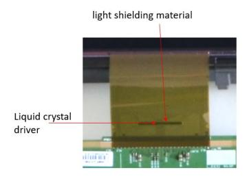
49. The products accused of infringing the '377 patent comprise a film carrier comprising said circuit pattern formed on a resin film. For example, an examination of LGD's TFT-LCD included in Heesung LCM model no. HC490EQH-SLXA1-211X demonstrates this:
