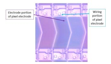
82. The products accused of infringing the '347 patent are configured such that the electrode portion is at least partially constituted by a transparent electric conductor. For example, the pixel electrode portion is at least partially constituted by a transparent electric conductor. For example, an examination of LGD's TFT-LCD included in Heesung LCM model no. HC490EQH-SLXA1-211X demonstrates this:
