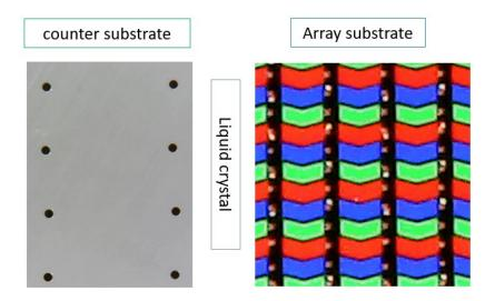
98. The products accused of infringing the '682 patent comprise a plurality of scanning signal lines and a plurality of video signal lines formed so as to define a plurality of pixels in a matrix on an inner surface of one of the pair of substrates. For example, an examination of LGD's TFT-LCD included in Heesung LCM model no. HC490EQH-SLXA1-211X demonstrates this:
