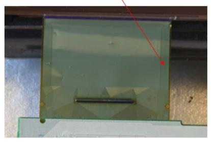
50. The products accused of infringing the '377 patent are configured such that the liquid crystal driver is mounted on the liquid crystal panel by a light shielding resin disposed on said liquid crystal panel so as to cover one end of the film carrier and a side surface of said liquid crystal driver. For example, an examination of LGD's TFT-LCD included in Heesung LCM model no. HC490EQH-SLXA1-211X demonstrates this:
