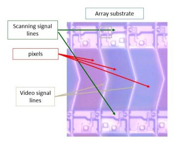
99. The products accused of infringing the '682 patent comprise a pixel electrode and a common electrode formed opposite to each other in each pixel in a plan view. For example, an
