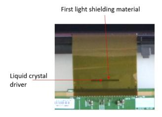
63. The products accused of infringing the '706 patent comprise a second light shielding material disposed adjacent an opposite face of said liquid crystal driver so as to prevent an outer light from being incident to said liquid crystal driver. For example, an examination of LGD's TFT-LCD included in Heesung LCM model no. HC490EQH-SLXA1-211X demonstrates this:
