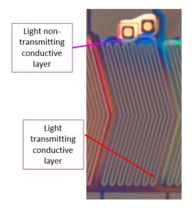
102. The products accused of infringing the '682 patent are configured such that a width of the light-transmitting conductive layer is wider than a width of the light-non-transmitting layer. For example, an examination of LGD's TFT-LCD included in Heesung LCM model no. HC490EQH-SLXA1-211X demonstrates this:
