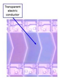
83. The products accused of infringing the '347 patent are configured such that the pixel electrode portion is formed in a layer separated by an insulating layer from a layer in which the scanning signal line is formed, and the pixel wiring portion is formed in the layer in which the scanning signal line is formed. For example, an examination of LGD's TFT-LCD included in Heesung LCM model no. HC490EQH-SLXA1-211X demonstrates this:
