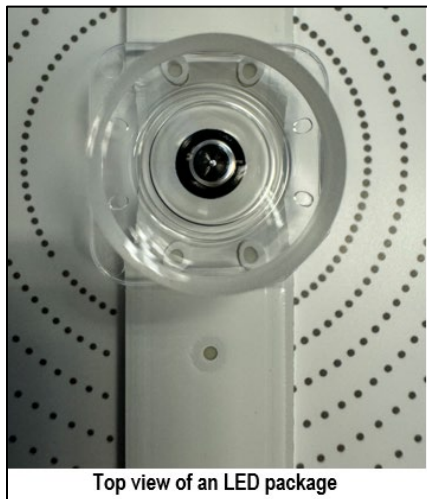
Top view of an LED package with lens removed
