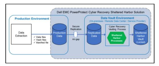
73. The Sheltered Harbor specifications require participants to protect critical data sets, including by creating dedicated, isolated environments which are physically separated from corporate networks and backup systems. Such data sets are converted for storage into Sheltered Harbor standardized
