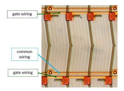
115. The products accused of infringing the '303 patent are configured such that the array substrate is provided with a common electrode being electrically connected to the common wiring and generating an electric field between the common electrode and the pixel electrode creating a voltage for driving the liquid crystal. For example, an examination of BOE's LCM/LCD model no. NV156FHM-N3D demonstrates this:
