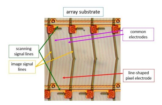
64. The products accused of infringing the '829 patent comprise a switching element for electrically connecting the pixel electrode and one of the image signal lines in response to a signal received from the scanning signal lines. For example, an examination of BOE's LCM/LCD model no. NV156FHM-N3D demonstrates this:
