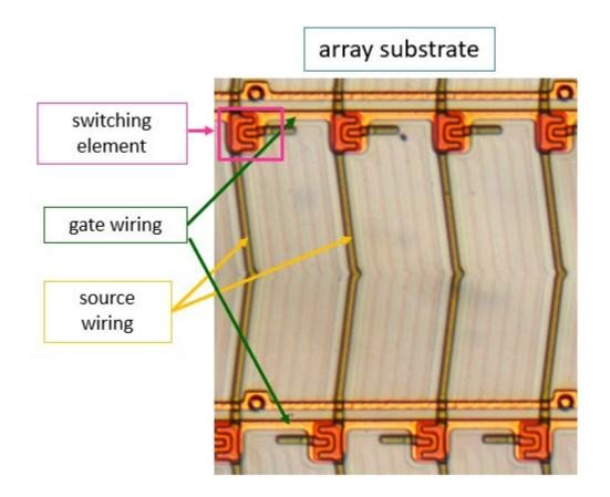
114. The products accused of infringing the '303 patent are configured such that the array substrate is provided with a common wiring formed between the two adjacent gate wirings. For example, an examination of BOE's LCM/LCD model no. NV156FHM-N3D demonstrates this:
