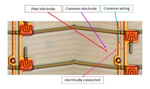
116. The products accused of infringing the '303 patent are configured such that the array substrate is provided with a storage capacity electrode electrically connected to the pixel electrode. For example, an examination of BOE's LCM/LCD model no. NV156FHM-N3D demonstrates this:
