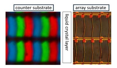
79. At least one of the substrates on the products made using the method of manufacturing accused of infringing the '293 patent includes pixel electrodes for generating an inplane electric field, common electrodes, and an insulating film for insulating these electrodes from one another. For example, an examination of BOE's LCM/LCD model no. NV156FHM-N3D demonstrates this:
