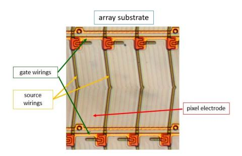
113. The products accused of infringing the '303 patent are configured such that the array substrate is provided with a switching element for switching a voltage applied to the pixel
