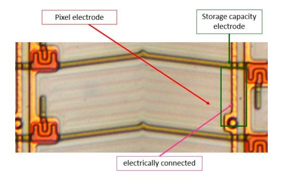
117. The products accused of infringing the '303 patent are configured such that the pixel electrode and the storage capacity electrode are layered so as to hold at least some part of the common wiring in between through an insulating layer. For example, an examination of BOE's LCM/LCD model no. NV156FHM-N3D demonstrates this:
