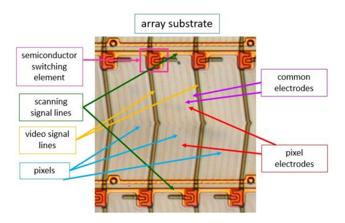
46. The products accused of infringing the '798 patent comprise a counter substrate arranged opposite the array substrate, and a liquid crystal layer sandwiched between the array substrate and the counter substrate. For example, an examination of BOE's LCM/LCD model no. NV156FHM-N3D demonstrates this:
