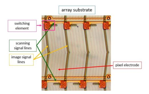
65. The products accused of infringing the '829 patent are configured such that of the pixel electrode and the common electrode, the electrode that is located adjacent to and parallel to one of the image signal lines or one of the scanning signal lines comprises an opaque conductor, and at least one of the other electrodes comprises a transparent conductor. For example, an examination of BOE's LCM/LCD model no. NV156FHM-N3D demonstrates this:
