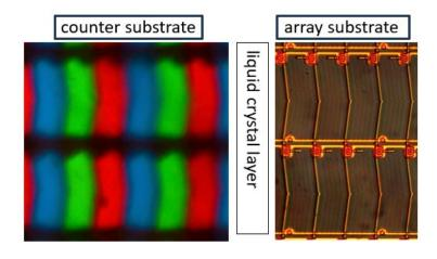
47. Each of the pixels in the products accused of infringing the '798 patent includes a plurality of electrode pairs, each electrode pair comprising one of the common electrodes and an adjacent one of the pixel electrodes, and at least one of the electrode pairs differs from other electrode pairs in a thickness of its common electrode or a thickness of its pixel electrode. For example, an examination of BOE's LCM/LCD model no. NV156FHM-N3D demonstrates this:
