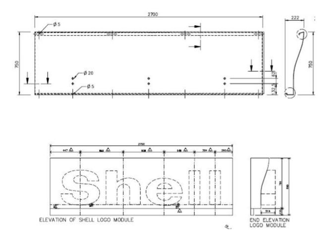
17. The curve of the Lazy S design itself is defined by two radii having a tangent point from one radii on one side of the fascia that is slightly offset from another tangent point of the other radii on the other side of the fascia as shown below:
