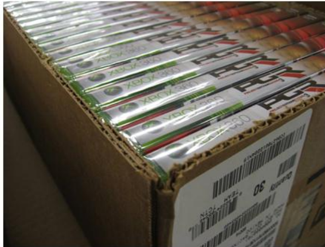
Example of tightly packed box opened by ABOT with correct cut depth and cut line settings
